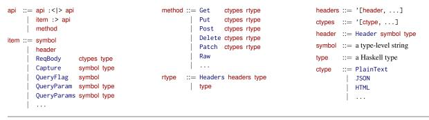
Figure 2. Grammar of the Servant type-level DSL for APIs
